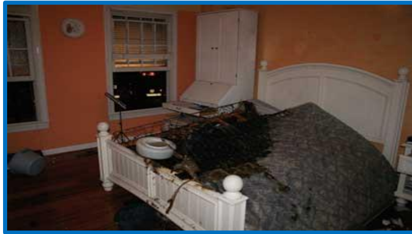
Figure 159 Bedroom fire that was extinguished with the activation of a Single Residential Sprinkler Head and virtually no damage to the room itself.
